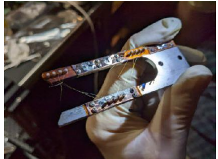
Wire scanner card halfway through a run
