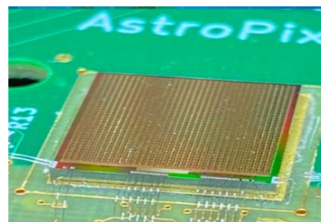
AstroPix tracking layers to capture 3D image of shower development NASA AMIGO-X mission
