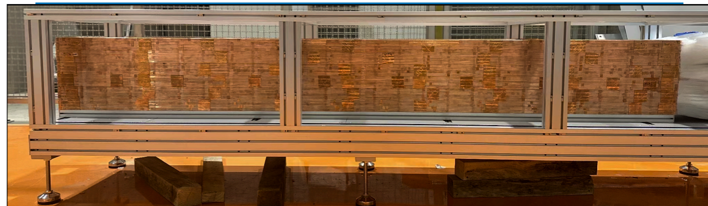
Figure 29: Barrel region of the dual-readout calorimeter, with a few towers highlighted for visualization purposes (left). Backside of one tower with the assembly of tubes and the support structure around them, forming one tower (right).
