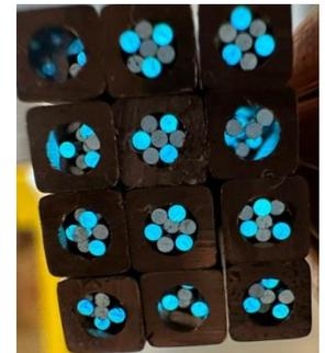
Individual towers ( $12 \times 16 \text{ mm}^2$ ) are constructed using fixtures
