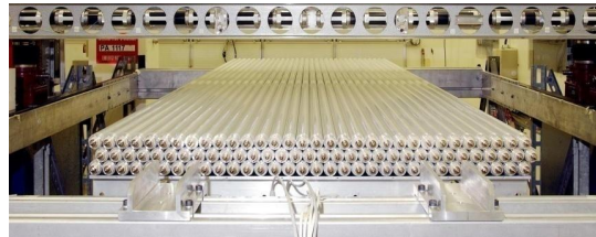
Muon MDT chamber, tube d=3 cm, 80 \mu m/wire
