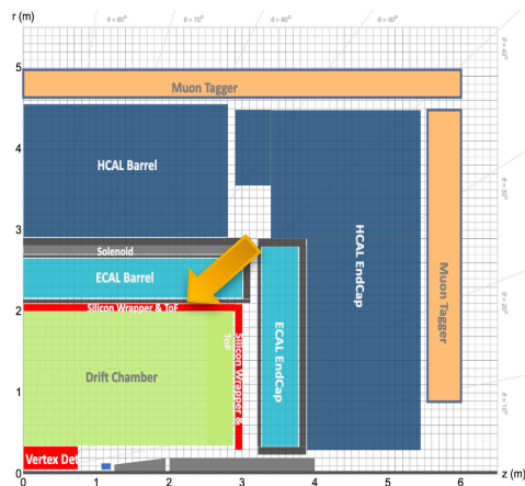
ALLEGRO Detector Concept (FCC-ee)
