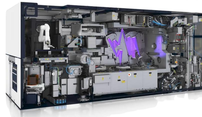
ASML's XUV lithography machine NXE:3400 for fabricating computer chips
