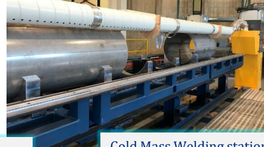
Cold Mass Welding station
