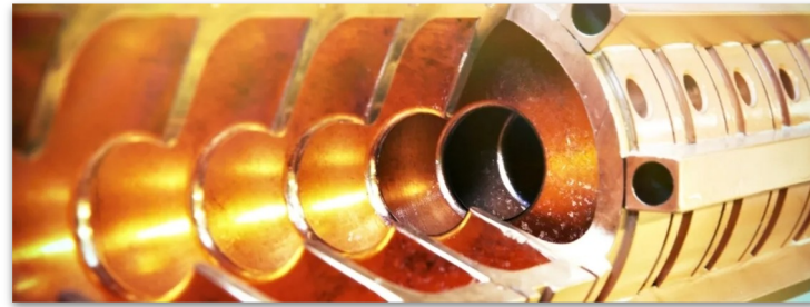
S-band copper RF structure
