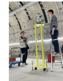
FIG. Total station measurement and calculation of the expanded control network
