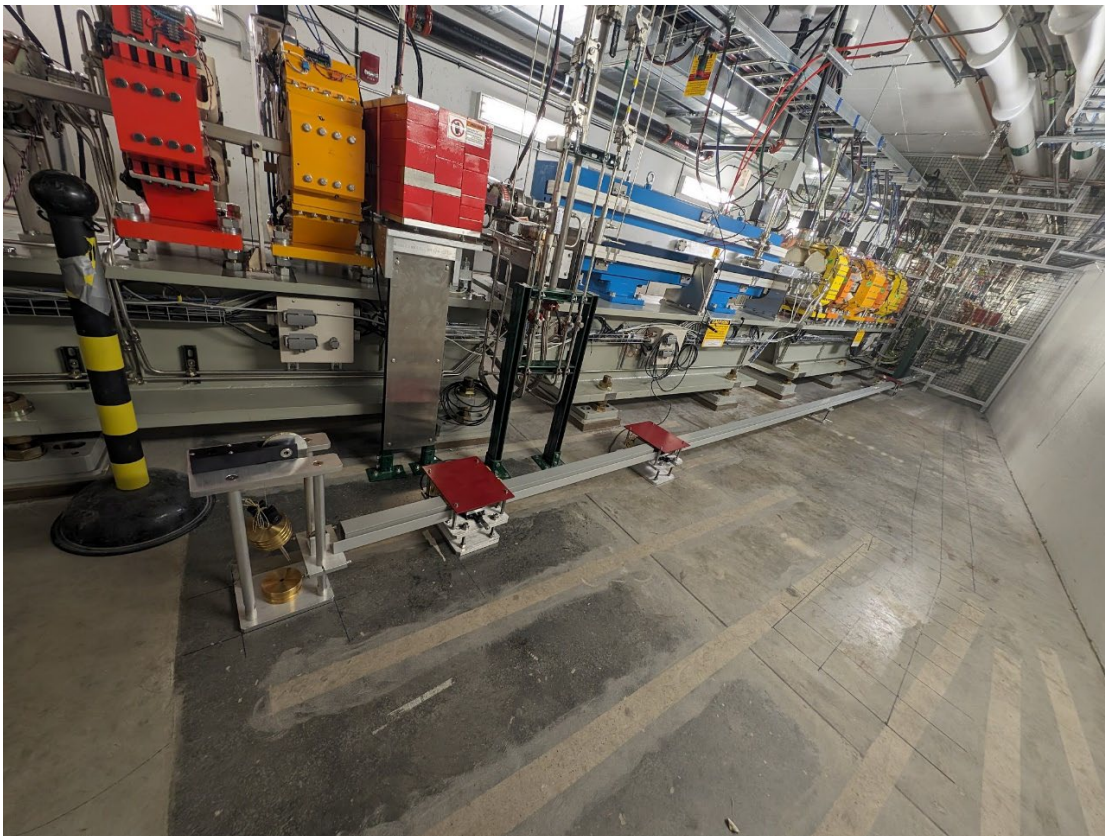
Figure 3: Monuments and instruments layout for monitoring floor changes above truck tunnel.
