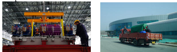
Fig.15 Girder Transportation Reliability Test
