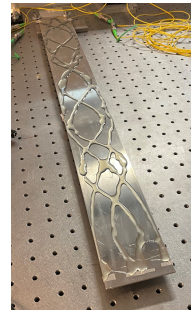
Figure 4: Steel plate, with 4 fibres glued on it. Each fibre has 6 splices and therefore measured sections.
