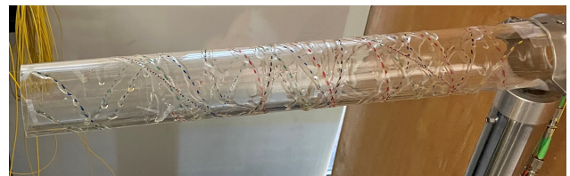
Figure 6: fibres glued on the surface of a Plexiglas tube.
