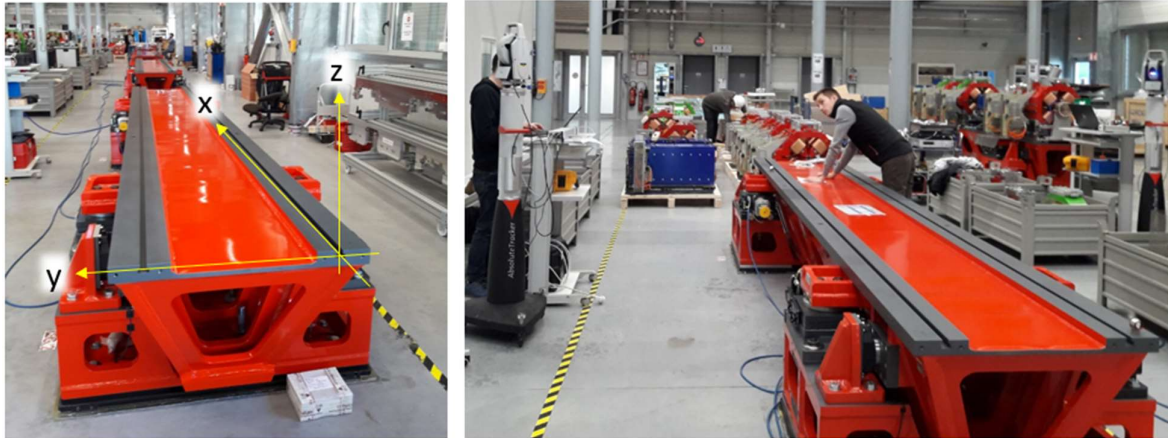
Figure 5 On the left the girder reference frame. On the right measuring the girder rectitude along the keyed surface.
