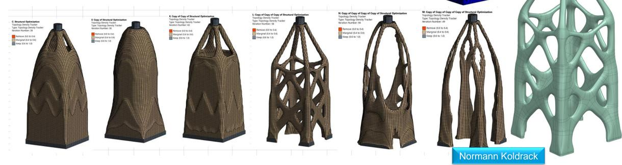
B: Modal Total Deformation 6 Type: Total Deformation
