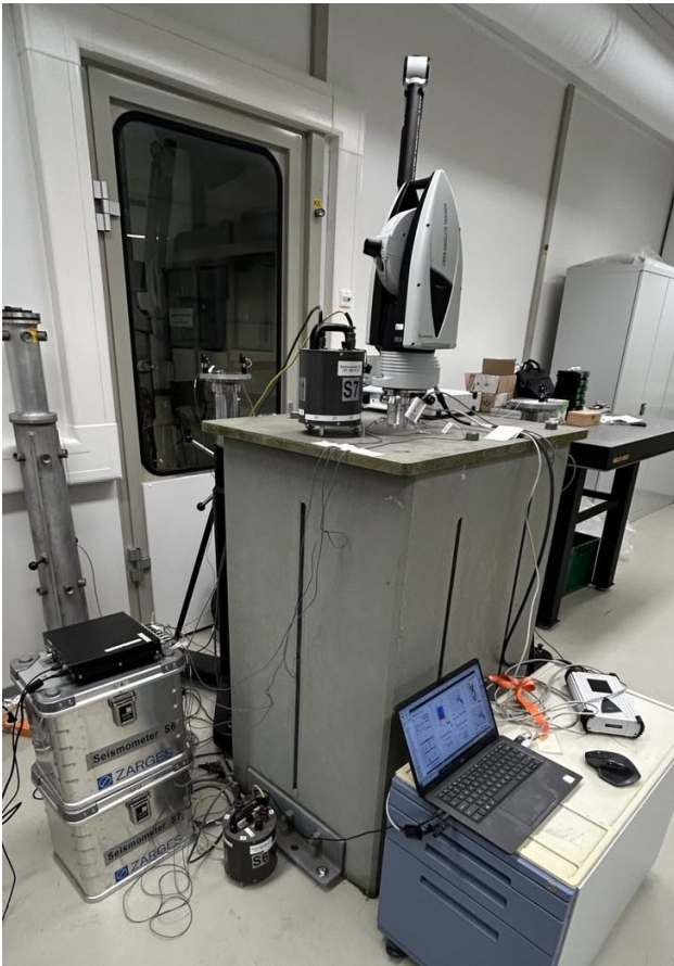
Figure 8: Testing of the concrete block pillar preprototype
