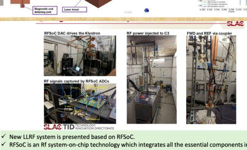
RFSoC is an Rf system-on-chip technology which integrates all the essential components including RFSoC based LLRF significantly reduces hardware complexity and enables more flexibility in operation They fabricated the LLRF based on RFSoC, and test it on pulse-to-pulse fluctuation, etc.
