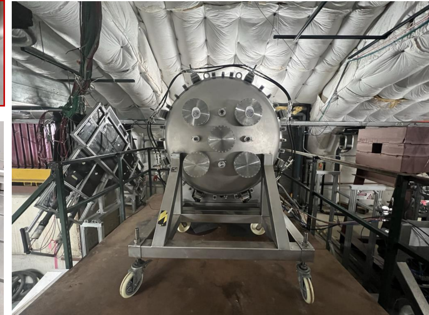
TOAD (Test of Overpressure Argon Detector) Beam test of readout chambers
