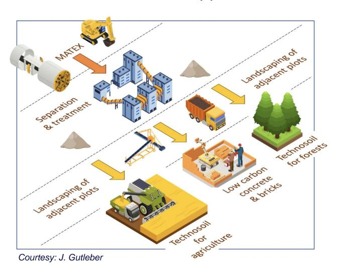
Excavated material from FCC subsurface infrastructures: 6.5 Mm<sup>3</sup> in situ, 8.4 Mm<sup>3</sup> excavated (bulk factor 1.3)
