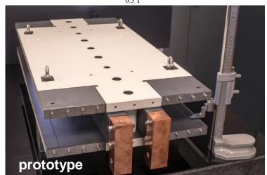
Twin F/D arc quad design with 2× power saving 25 MW (at 175 GeV), with Cu conductor
