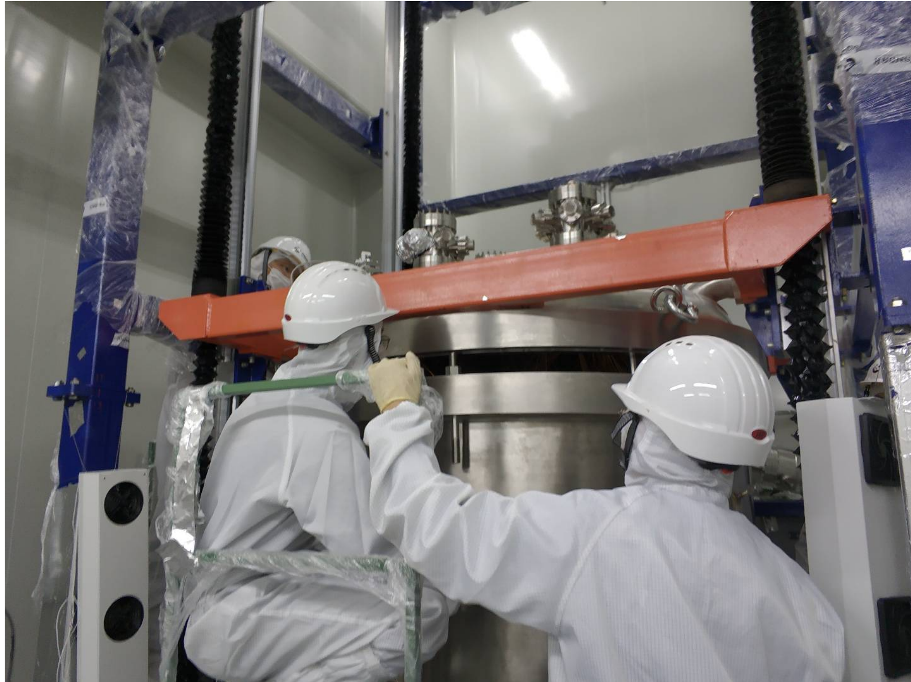
closure of the inner vessel
