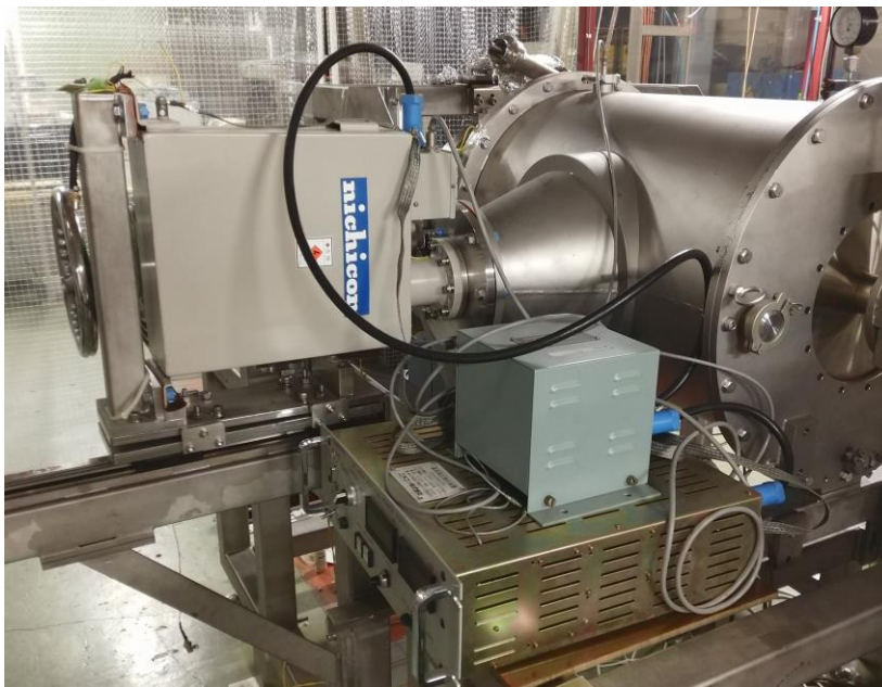
250 kV high-voltage power supply for spin-polarized electron gun
