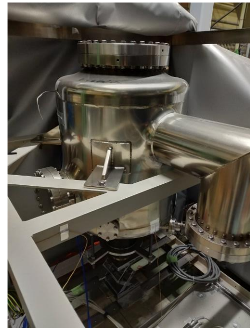
A large UHV chamber made of titanium
