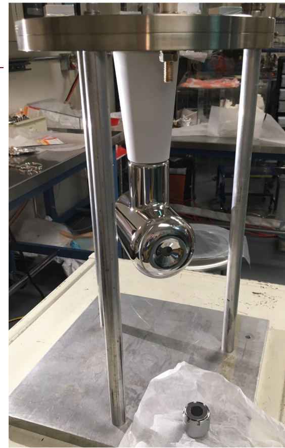
200 kV insulator for ILC/CEBAF
