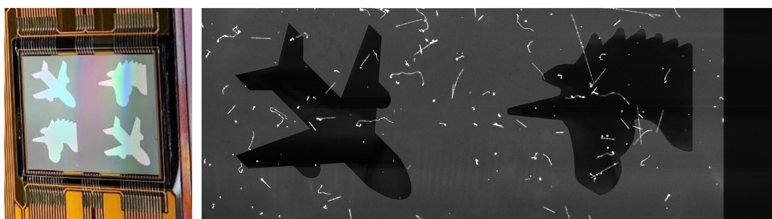
Figure 2: Skipper-CCDs with 50 nm Al shield. (Top) Picture of the sensor with Al layer covering half of the active area. (Left) same with an aluminum plane- and unicorn-shaped Al layers. (Right) Image acquired using the CCD upper half after illuminating 30 seconds with and LED.
