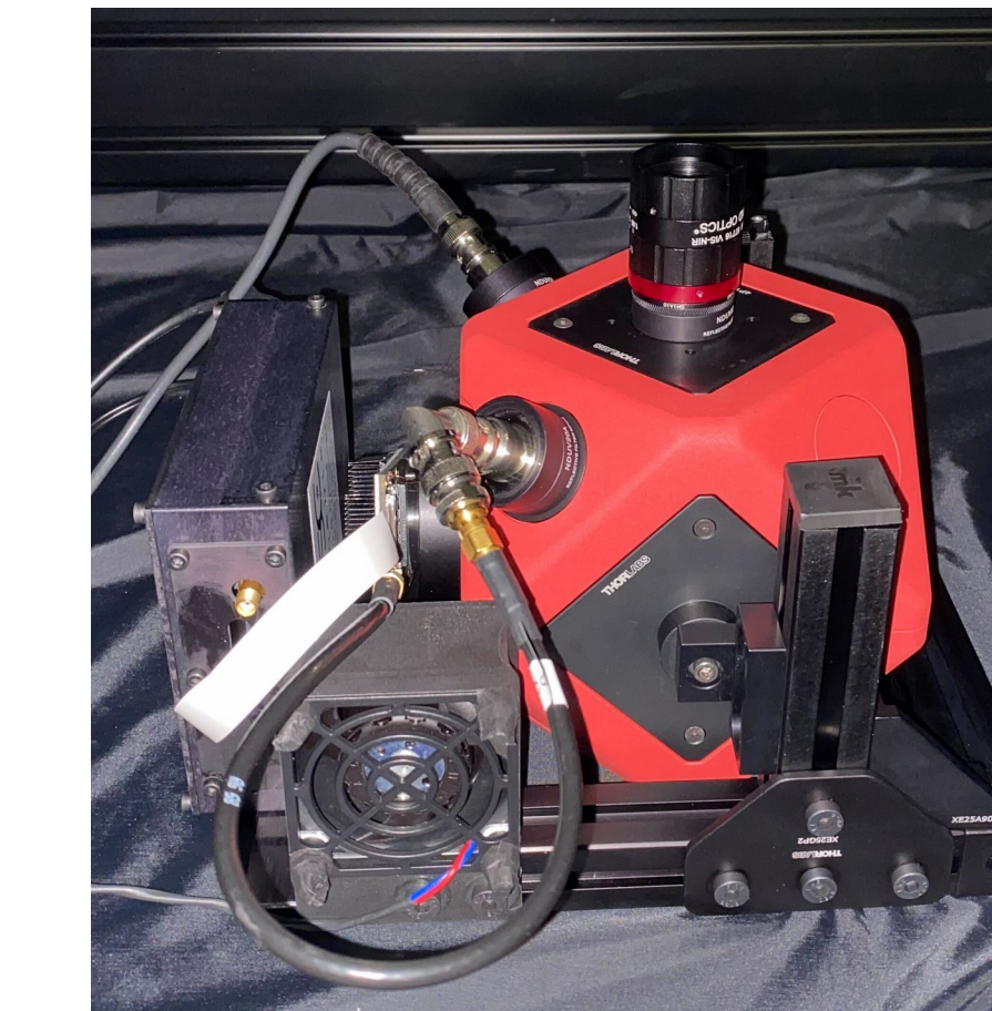
Figure 3: The wide beam projector used to create flat illumination across the entire focal plane.
