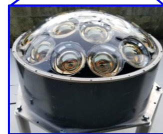
~102 mPMT modules x19, 3" PMTs each
