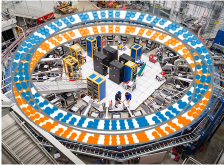
Fixed probes above/below muon storage region
