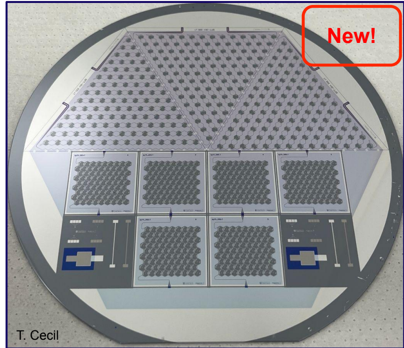
1/4 filled triangular subarrays for 3 bands Argonne 150mm wafer
