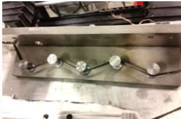
Interior of Impregnation Chamber
