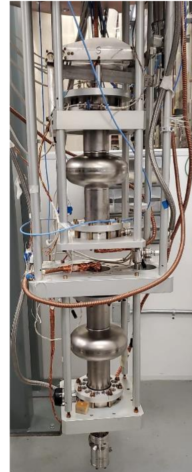
The experimental setup for the Dark SRF experiment consisting of two 1.3 GHz cavities
