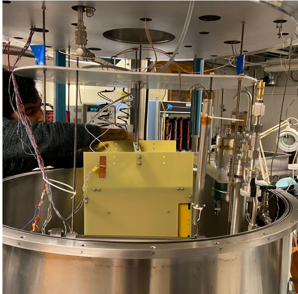
High Purity test stand at LBNL with SingleCube 30cm drift LArPix TPC
