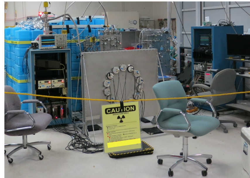
LLNL setup for LXe Migdal measurement, arXiv:2307.12952
