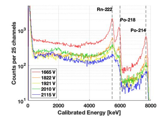
Calibration with radon source sample using alphas
