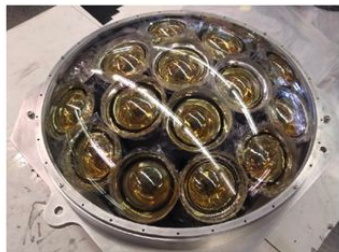
19 8cm PMTs in each mPMT module
