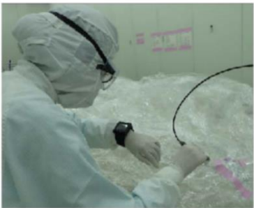
③ He leak test + repairs
