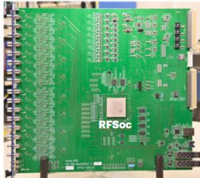
Deadtime free electronics (RFSoc) for better neutron capture tagging
