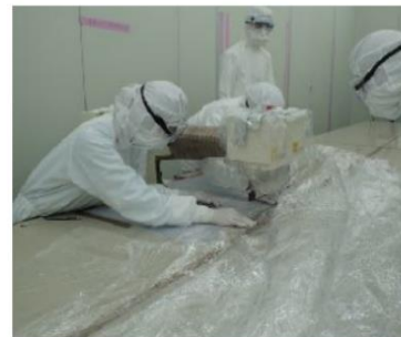
② Seam Welding
