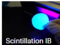
Scintillating Inner Balloon Film for better tagging of film backgrounds
