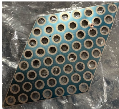
DLC coating electrode (150MΩ/mm 2 )
