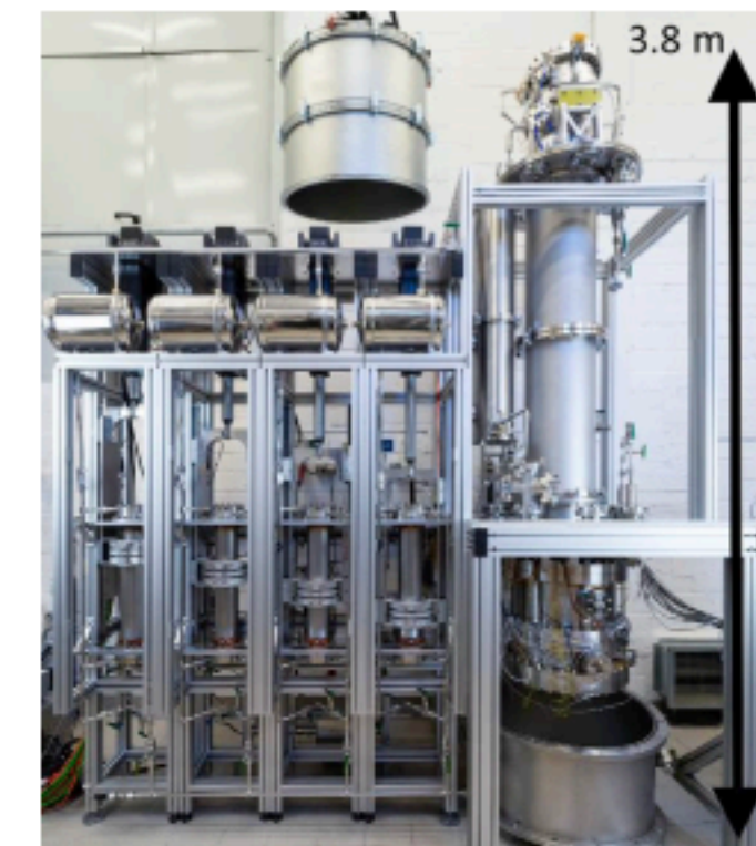
Rn distillation column for XENONnT (reduce ^{222}\text{Rn} - hence also ^{214}\text{Bi} - from pipes, cables, cryogenic system)
