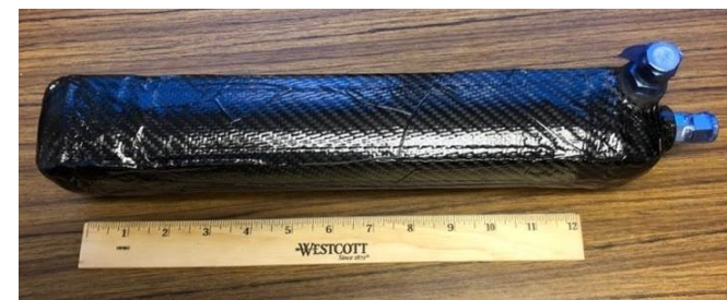
Full-size laminate adsorbent bed with SBMOF-1 adsorbent
