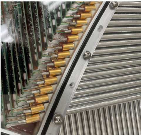
Front side of a preamp. Each preamp serves two straws
