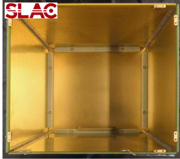
Cathode (bottom) and field cage
