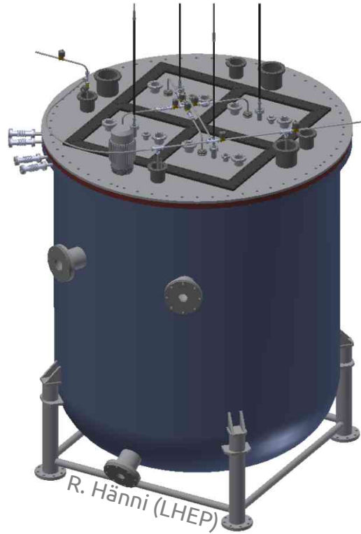
2x2 cryostat hosting four Module-0 like detectors
