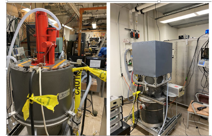
C-band klystron from SLAC recommissioned at MOTHRA. SLED system development this year.
