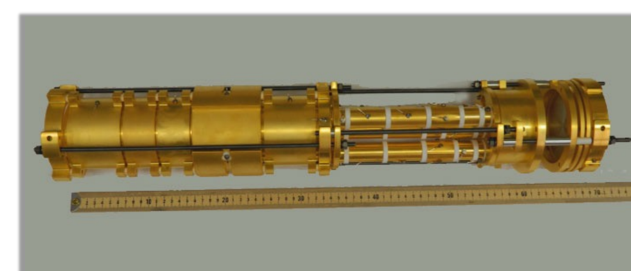
A multiplexed positron trap designed by the Surko group at UCSD. N. Hurst et al. Phys. Plasmas (2019)
