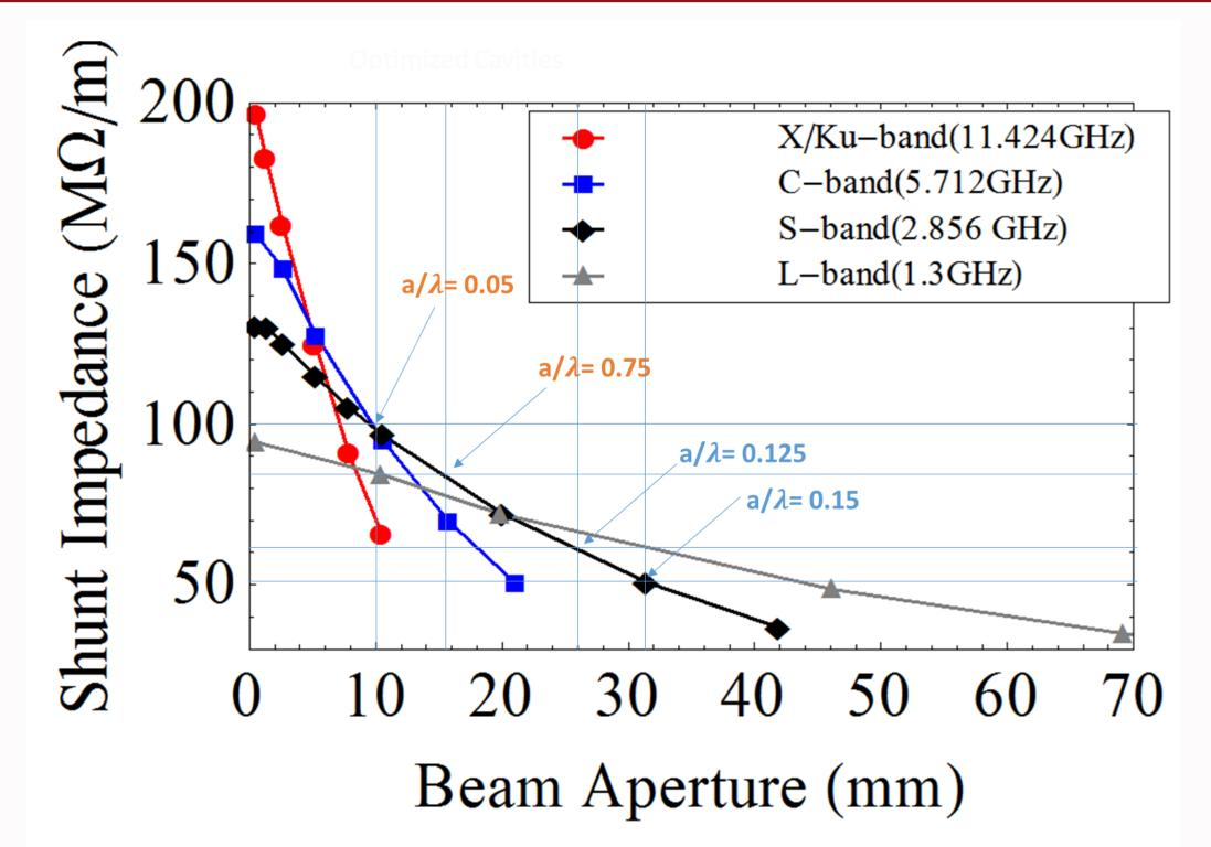
S-band cavities with a reentrant cell design feature a good balance of aperture radius and shunt impedance.
