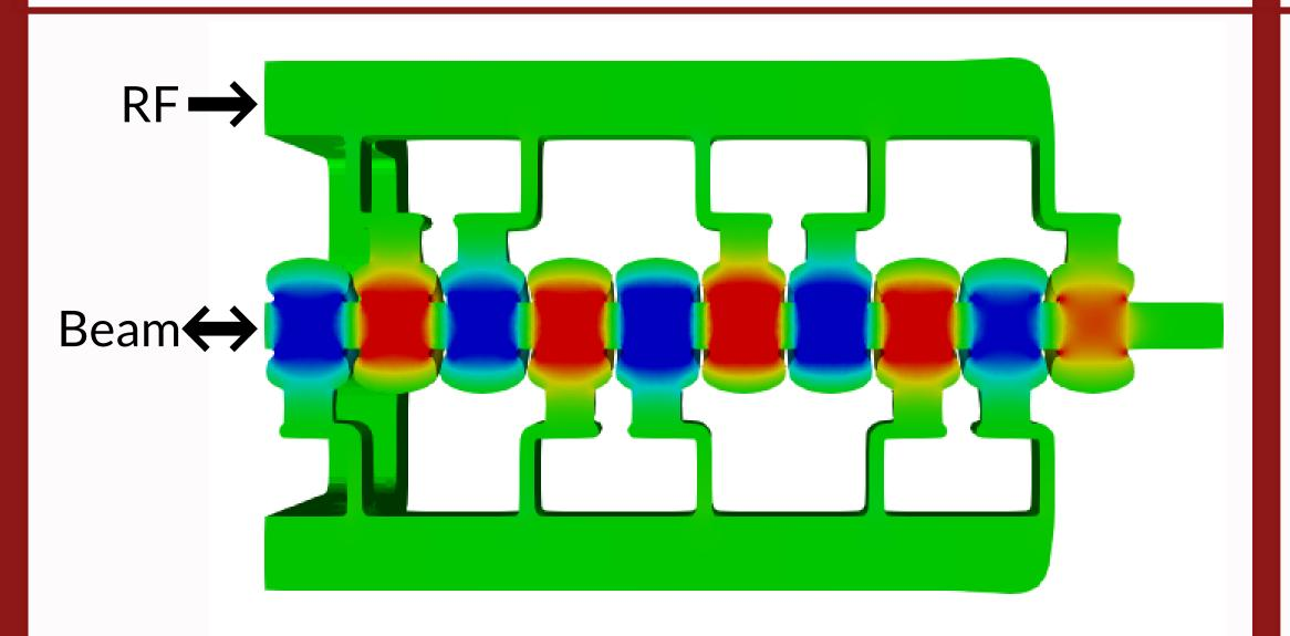
Distributed coupling uses unique waveguide and coupler design to power each cavity individually [2].
