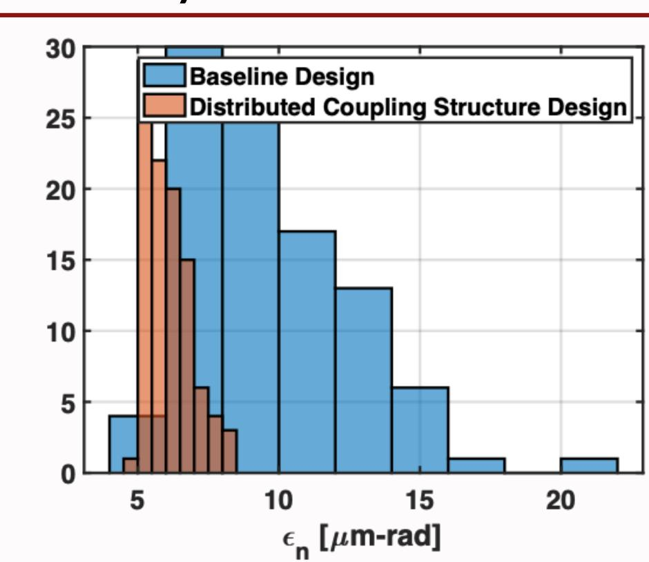
Compared to baseline traveling wave structures, our design maintains better output emittance for 14 nC bunches.
