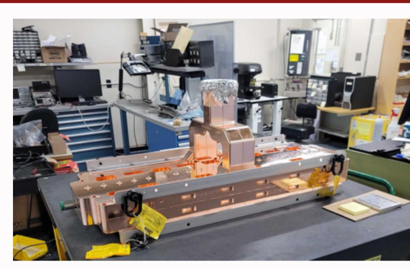
Assembly of one structure is complete, with tuning of field flatness underway.
