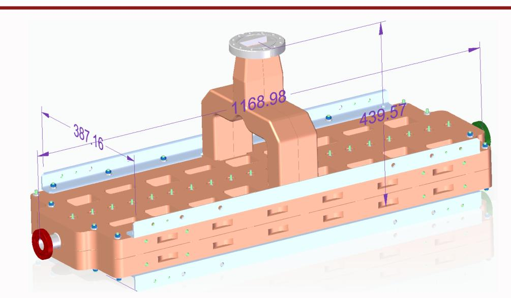
Current design uses two slabs to form the vacuum region in a meter-long structure, with a Y-coupler to distribute power.
