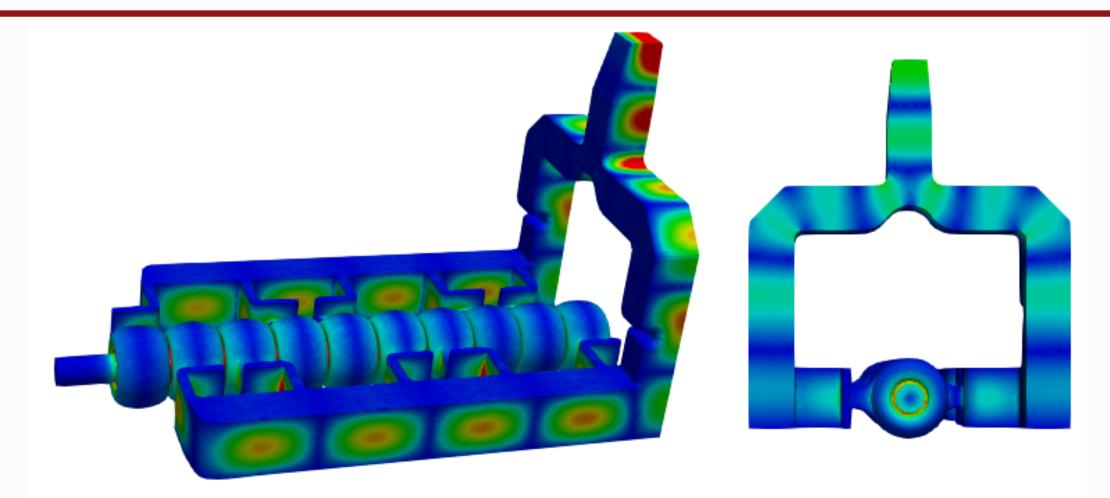
Simulations in HFSS and ACE3P verify the distributed power, with a  $\pi$  phase shift between successive cavities [3].
