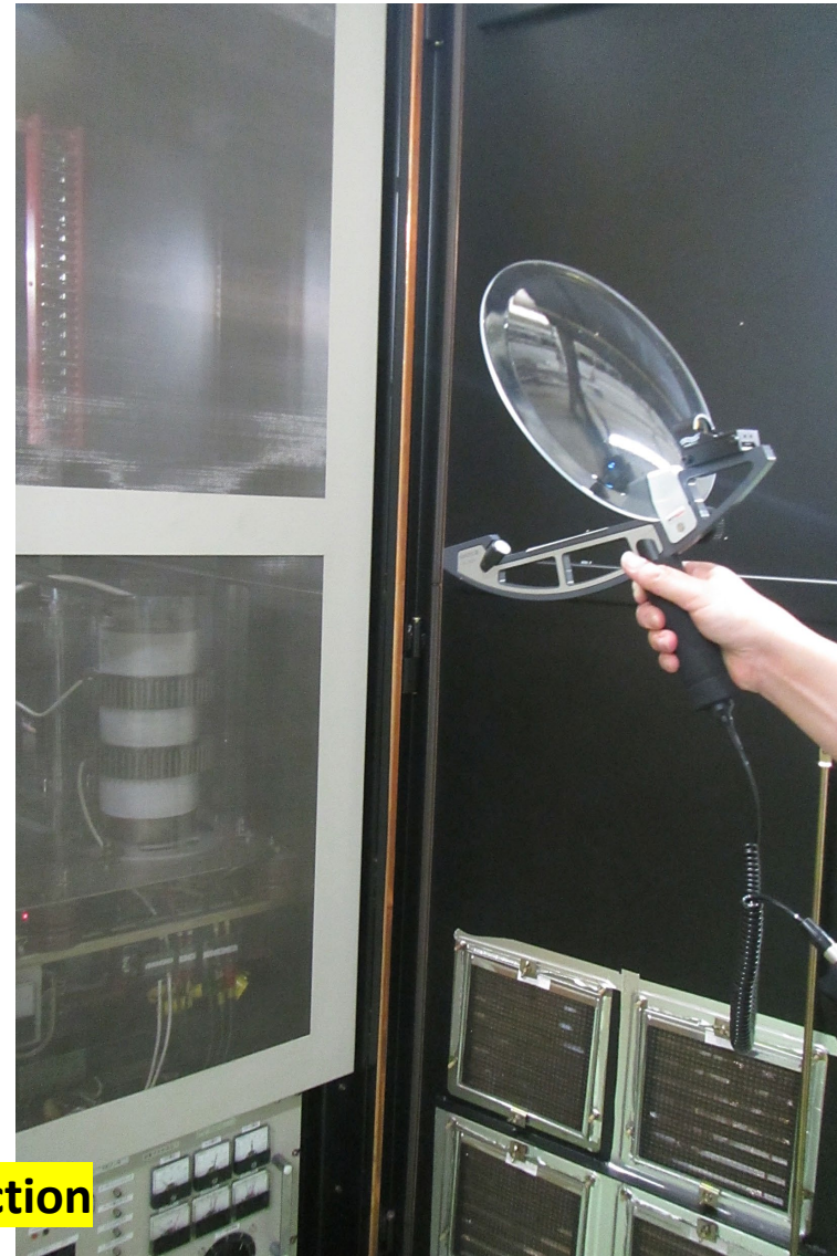
Ultrasonic leak detector made by SONOTEC Co., Ltd. (sensitive to \sim 40\text{kHz} )
