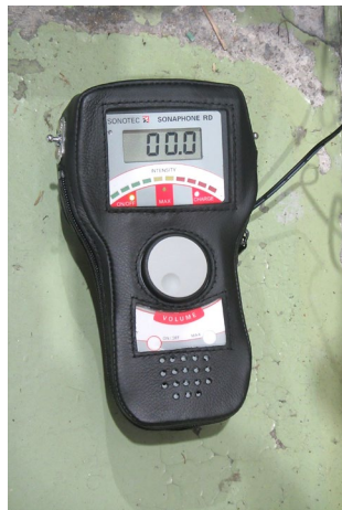
Ultrasonic leak detector made by SONOTEC Co., Ltd. (sensitive to \sim 40\text{kHz} )
