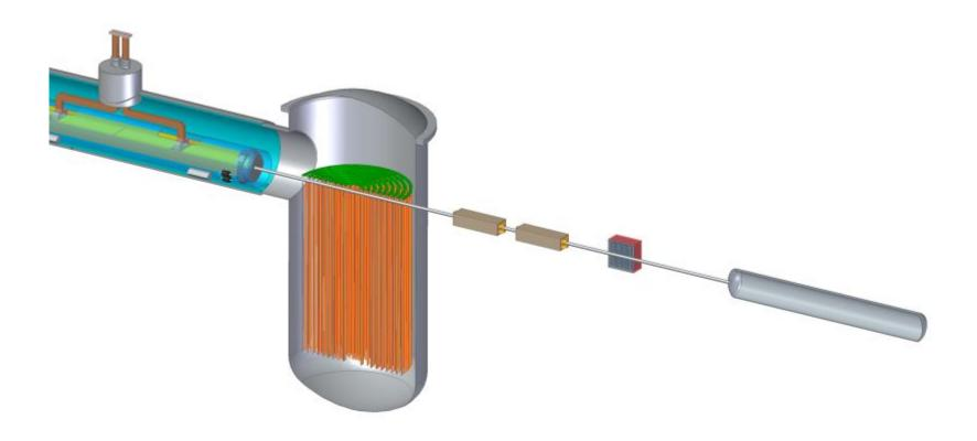
900 Calrods, 4 W/cm<sup>2</sup>, ~2 MW total. LN in boiler at same level as in cryomodules, covering Calrod array.
