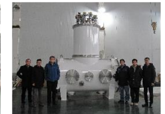
Horizontal test cryostat
