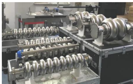
IHEP 1.3 GHz 9-cell Cavity Vertical Test
