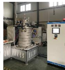
Nb 3 Sn furnace
