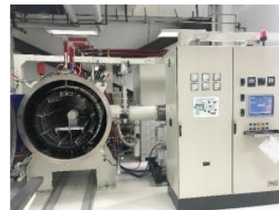
Vacuum furnace (doping & annealing)
