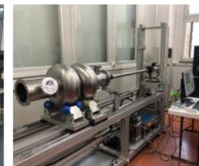
Cavity inspection camera and grinder
