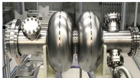
Vertical test of 650 MHz 2-cell cavity
