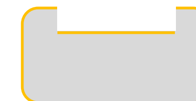
Groove machined by Turck head
