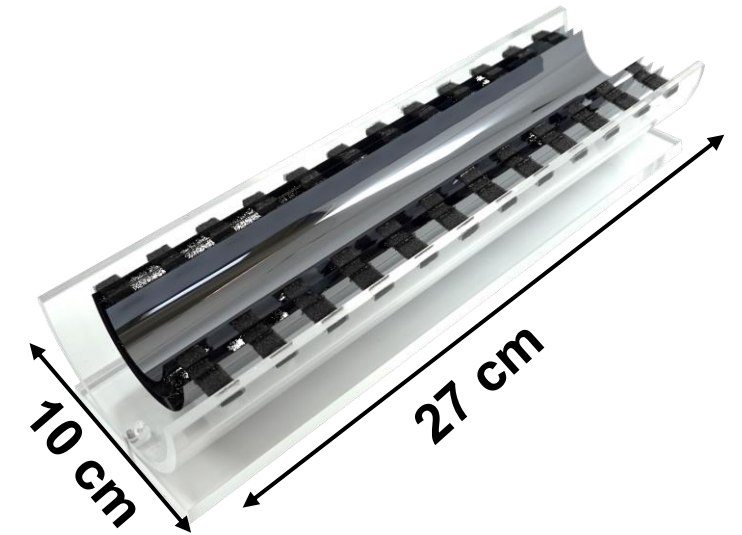
Large Area, Bent, Stitched Sensor, in the framework of R&D for ALICE ITS3
