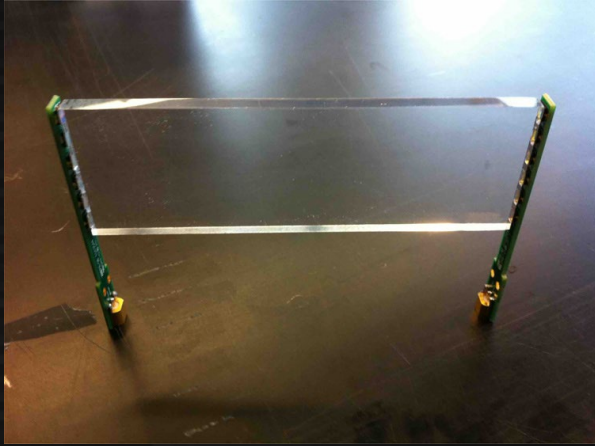
MEG2 timing counter (Plastic scintillator + 6 SiPMs) 40 psec achieved
