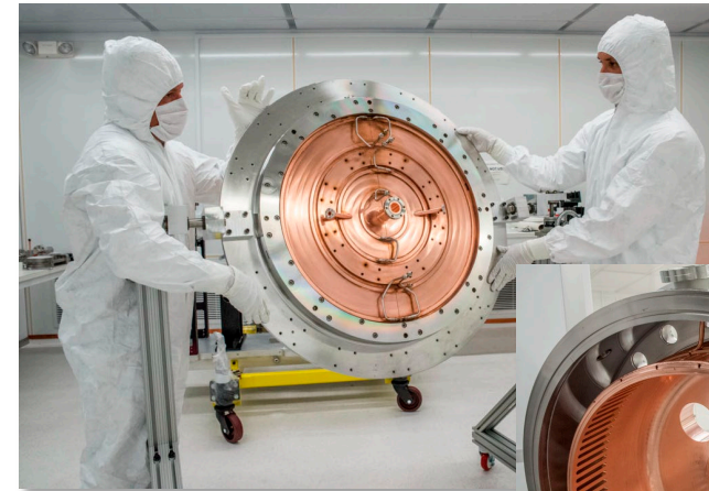
Electron Gun cavity
