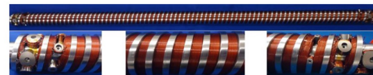
Superconducting helical undulator at Argonne, M. Kasa et al. Phys. Rev. Acc. Beams (2020)
