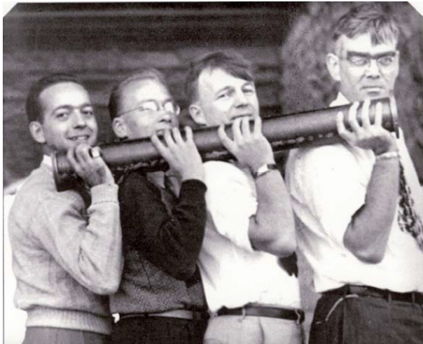
First 3-foot section of MARK I electron linear accelerator at Stanford (William Hansen and three of his students) 1947.
